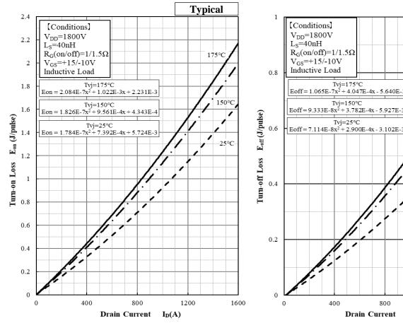
Turn-on Loss vs. Drain Current
