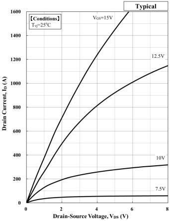
Drain Current vs. Drain - Source Voltage
