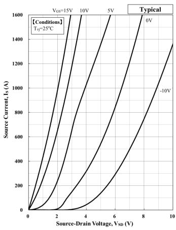
Source Current vs. Source - Drain Voltage
