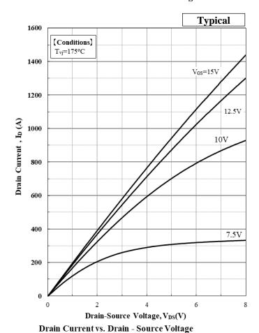
**Typical** 1600 [Conditions] V<sub>GS</sub>=15V  $T_{vj}=150^{\circ}C$ 1400 12.5V 1200 Drain Current, I<sub>D</sub> (A) 1000 10V 800 600 400 7.5V 200 Drain-Source Voltage, VDS (V)
